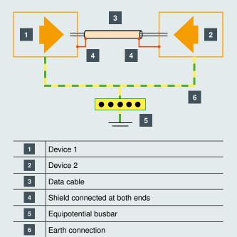
Cable shield earthed at both ends
